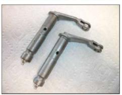
The above photo shows a pair of brake levers with grease fittings installed. Drill from the end of the shaft with a nominal 1\8" drill bit down to a point between where the two bushings ride and cross drill it. Then drill the end of the shaft with a 5\16" drill bit about 3\8" deep.
