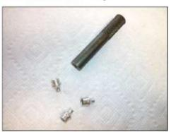
Press in type grease fittings and the insertion tool
